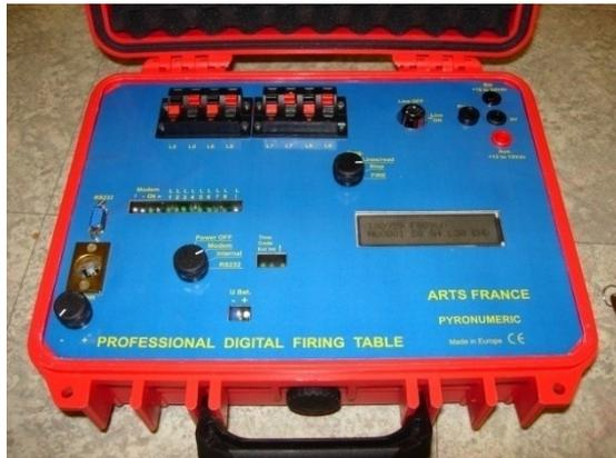
This machine functions by using the same equipment (receivers & power station) and by following the same process as the manual table. It replaces the 960 firing table and gives you much more: up to 4000 lines programmed to 1/10<sup>th</sup> of a second (or to 1/20<sup>th</sup> by using 32 sequencers), which can be transformed into 4000 x 32 = 128 000 lines set up wherever you chose by adding 32 programmed sequencers.
